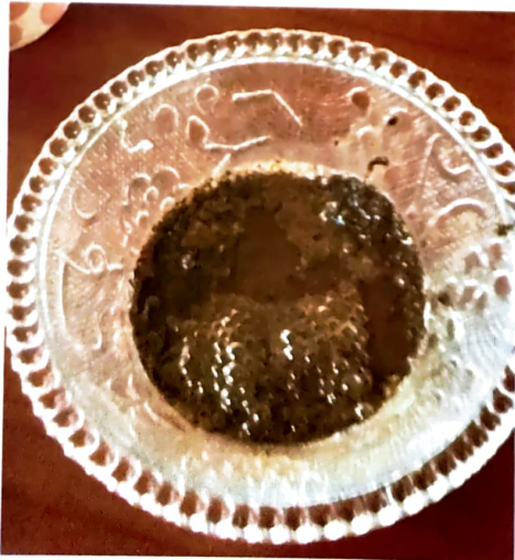
Figure 1: Soil sample showing fizzing reaction with vinegar. Thus, it is Alkaline soil.
