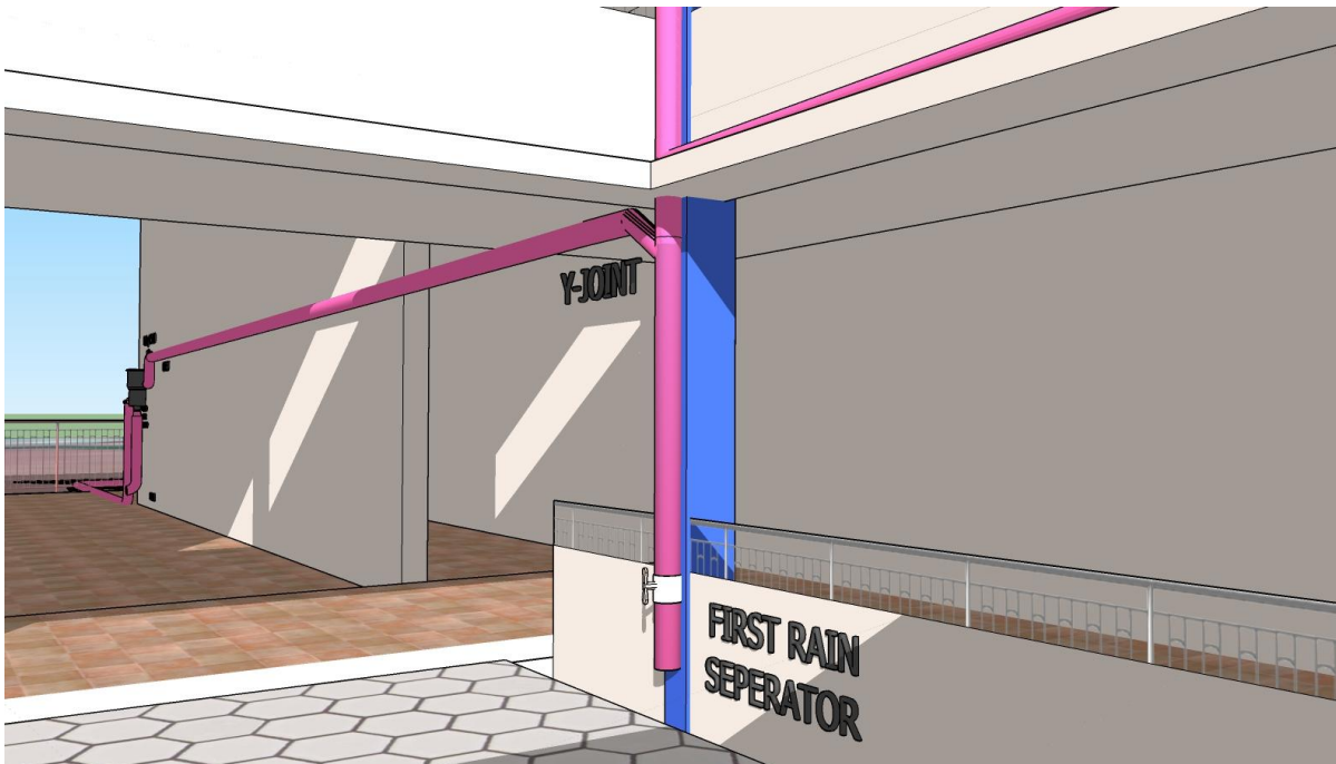
Fig : First rain separator and Wall mountable rainwater filter
